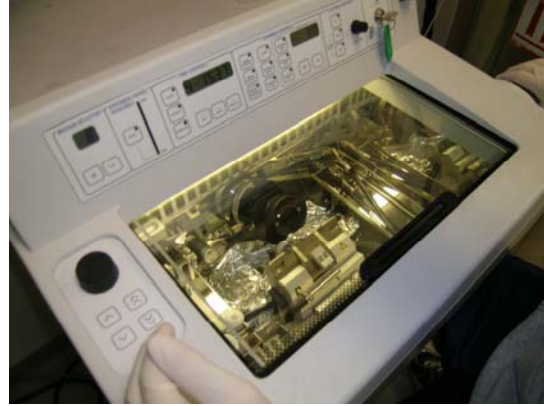
Figure 4a: Cryosectioning machine (outside)
