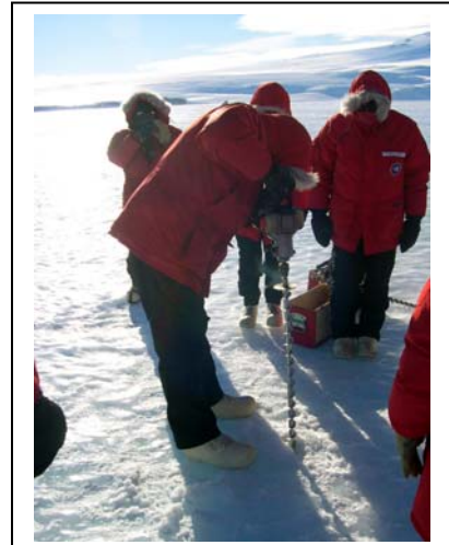
Drilling to determine the ice thickness at Sea Ice School.
